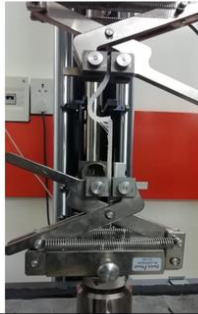
Fig4: The visual examination of peeling of silicone from the acrylic samples
