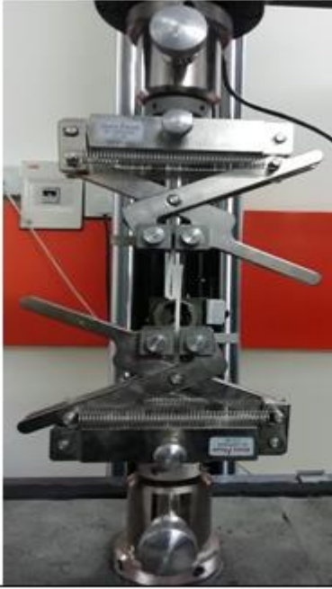
Fig3: The unbound silicone is turned back at 180° and gripped in upper clamp
