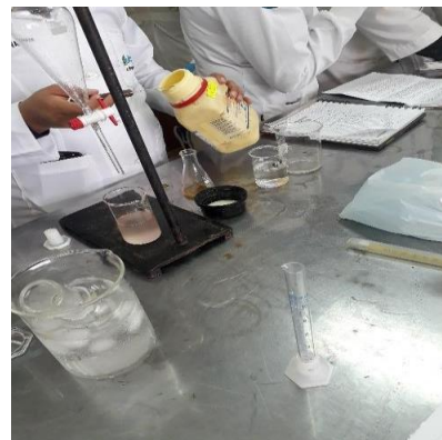
Figure 3.6. Release of \text{CO}_2 from the organic phase after adding bicarbonate to the solution.
