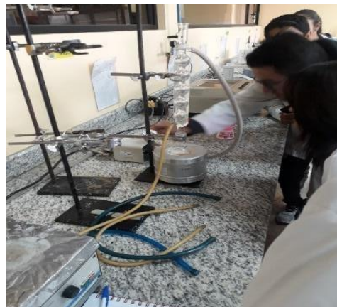
Figure 3.1. Stirring process without heating 5.3 mL of isoamyl alcohol with 7.3 mL of acetic acid.
