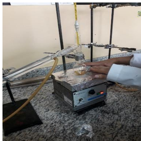
Figure 3.7. Magnetic stirrer placed in the solution in the distillation process.
