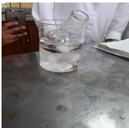
Figure 3.4. Cooling of the solution in a water bath and an ice bath.
