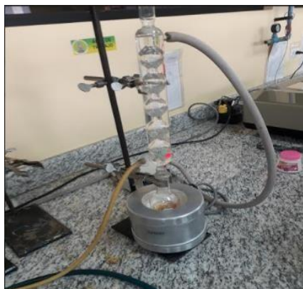
Figure 3.3. Reflux of organic material in the presence of sulfuric acid by heating
