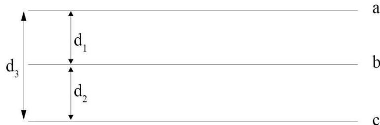
Figure 14: A diagram showing how the three conductors of a 3-phase transmission line are separated from each other
