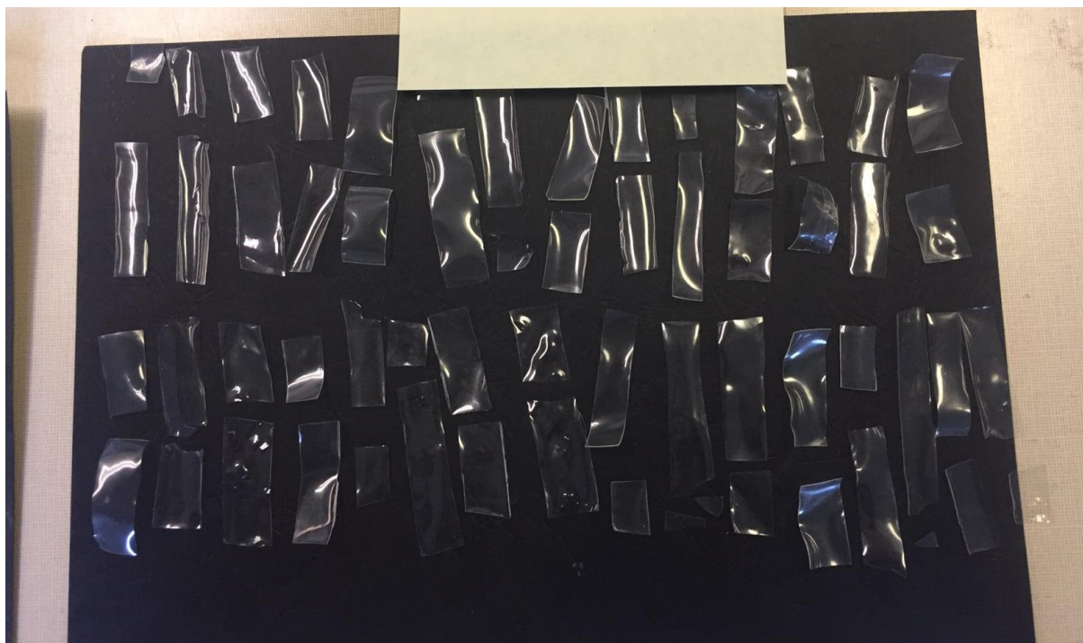
Figure3 . Broken solvent-based epoxy coating samples after tensile stress test
