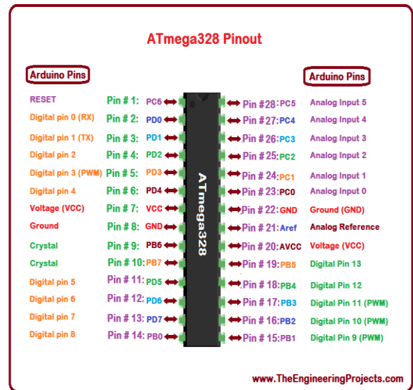
Fig. 5: The Pin-out of ATmega328P Microcontroller
