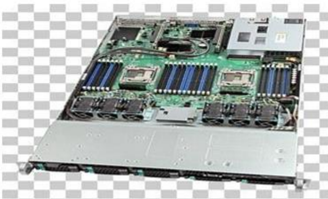
Figure.5 : Inside view of the Intel server.
