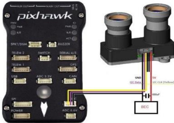
Figure 17: LIDAR Connections to PIXHAWK
