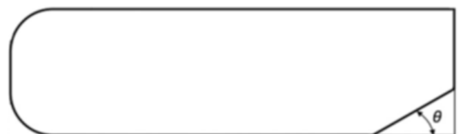
FIGURE 4. INVERTED AHMED BODY ADAPTED AS A DIFFUSER BLUFF BODY
