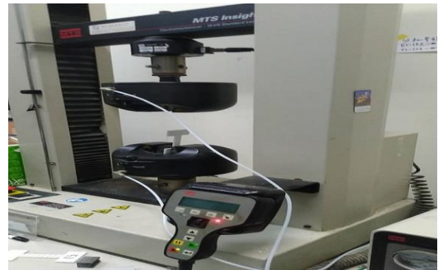
Fig. 11. Specimen and tensile testing module
